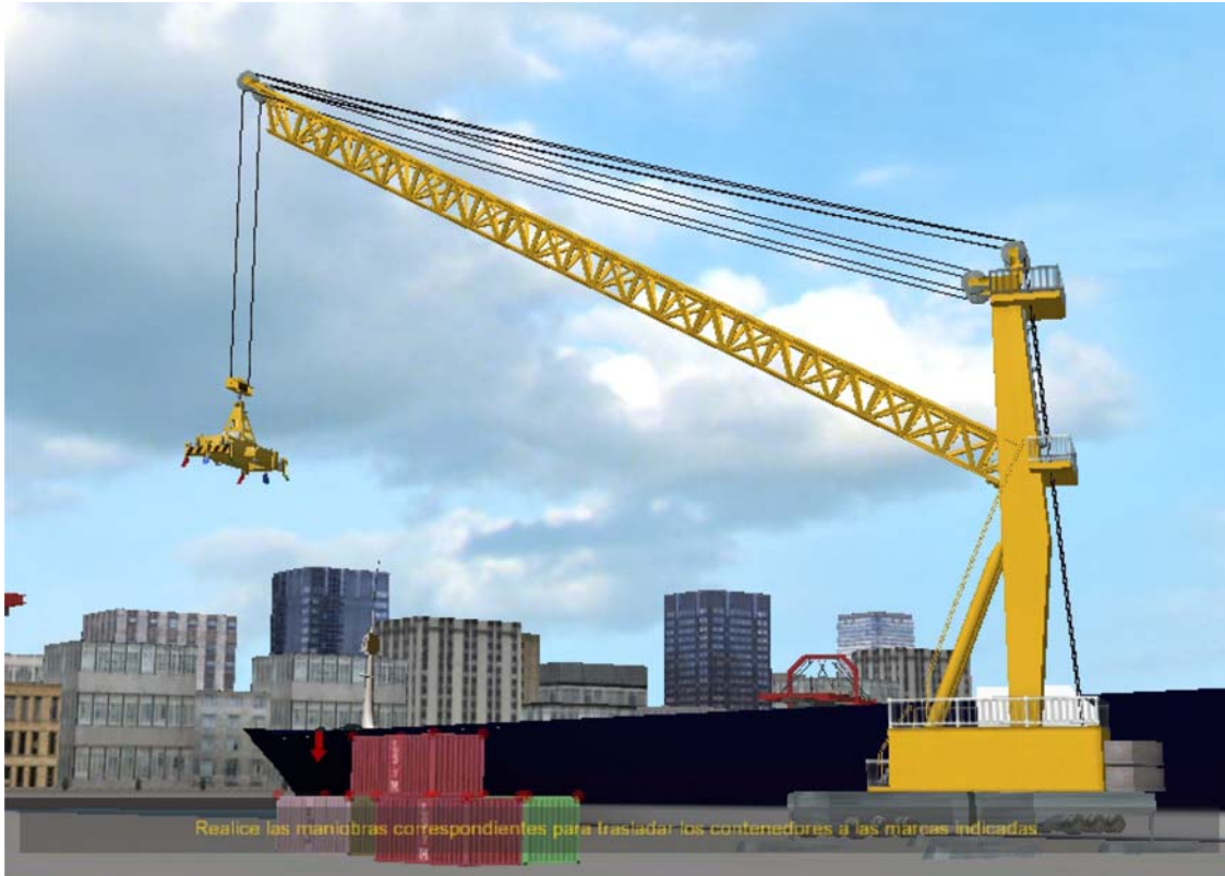
Figure 8 Cable and pulley systems are often present in harbour cranes. A mobile crane usually uses this kind of system to hoist the load and also for the movement of the boom (see online version for colours)
