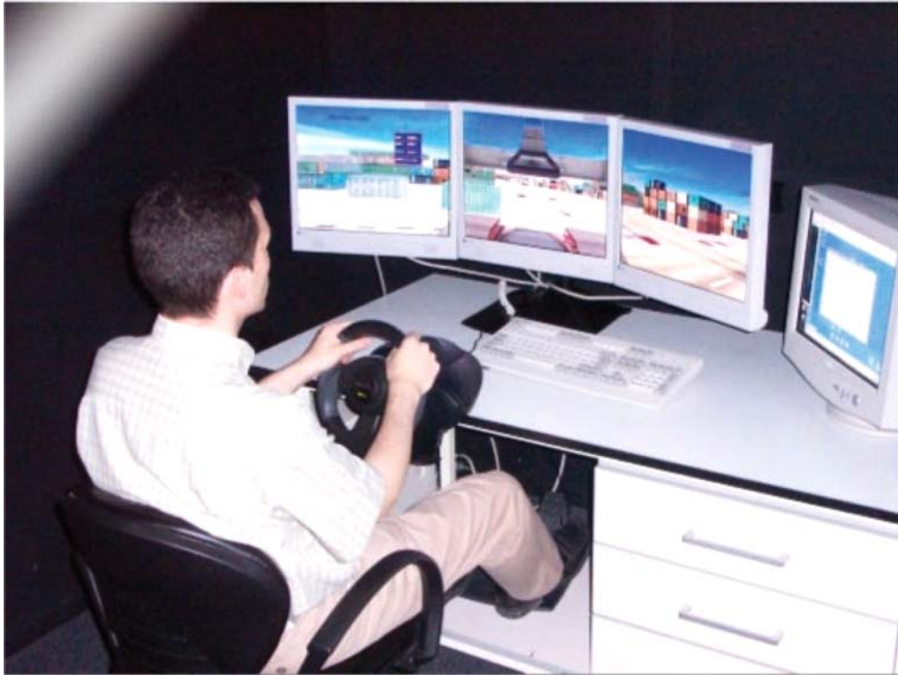
Figure 10 A desktop configuration, with several displays and conventional game devices used as crane controls (see online version for colours)
